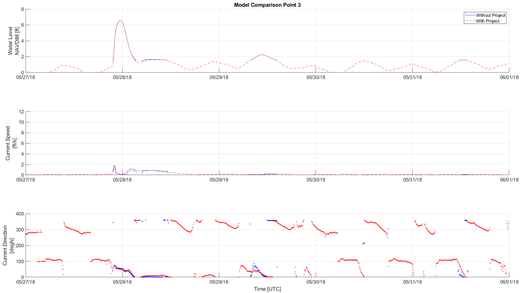
Figure B-21: Modeled with project (red) and without project (blue) project hydrodynamics during 100-year RP at model comparison point 3
