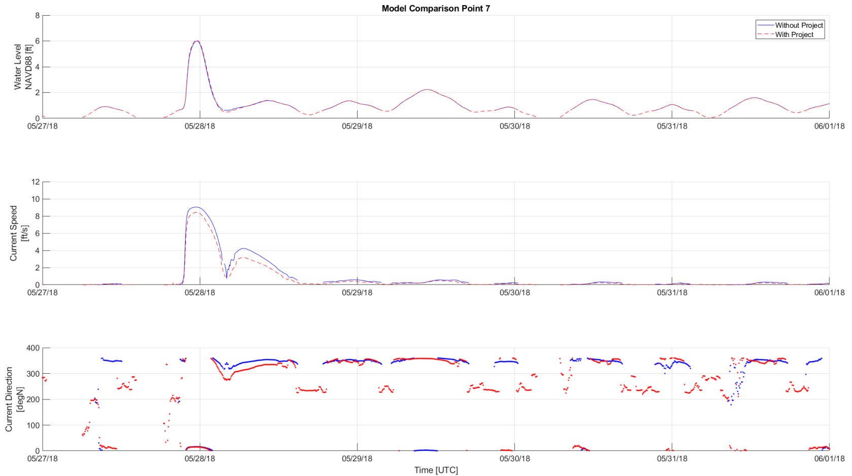
Figure B-25: Modeled with project (red) and without project (blue) project hydrodynamics during 100-year RP at model comparison point 7
